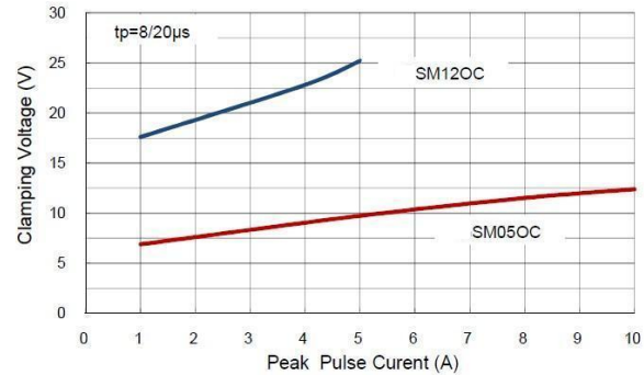
Fig 4 Peak Pulse Current vs Clamping Voltage
